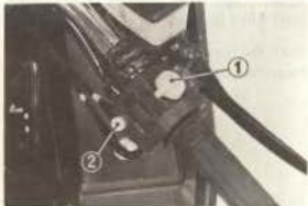
(1) Engine stop switch (2) Starter button
