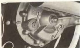
(1) Oil filler cap (2) Oil drain plug
