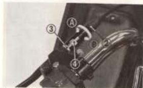
(2) Dust cover (3) Lock nut (4) Clutch cable adjuster
