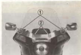
(1) Rear view mirror screws (2) Front panel screws
