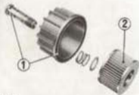
(1) O-rings (2) Oil filter element
