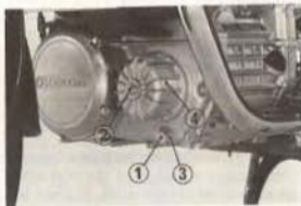
(1) Oil drain plug (3) Sealing washer (2) Oil filter bolt (4) Oil filter cover
