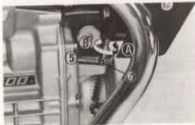
(5) Lock nut (A) Increase free play (6) Adjusting nut (B) Decrease free play
